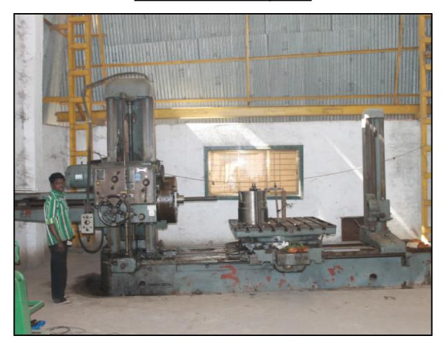
We have installed WMW make Horizontal Boring Machine at Bay# 5
